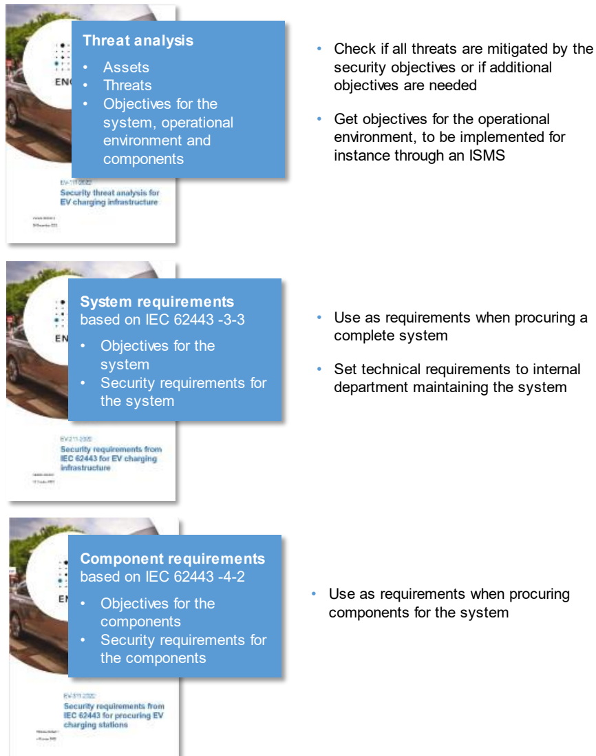
Figure 1: Relation between the different documents on EV charging infrastructure security.
